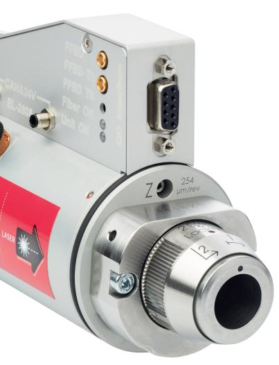
The Optoskand incoupling optics distributes the energy from a laser into one or several process fibers. The system can accept either a free space collimated beam from a laser or a feeding fiber from a fiber laser. It is possible to both time share or energy share a laser source between several work stations. Integrated control and safety electronics guarantee laser safety for the fiber beam delivery.
