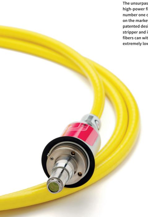
The unsurpassed performances of the Optoskand high-power fiber optic cables make them the number one choice for most industrial lasers on the market. Thanks to a well developed and patented design featuring quartz block, mode stripper and internal direct water cooling, the fibers can withstand high power levels and offer extremely low transmission losses.
